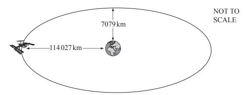
The height of satellite *NORAD 25989* is between 7079 km and 114027 km. It has an orbit time of 2872 minutes.
